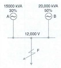
The percentage reactance of each alternator is based on its own capacity. Find the short - circuit current that will flow into a complete 3 - phase short - circuit at F.
